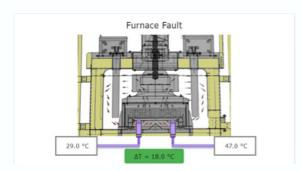
• THERMODYNAMIC CONDITION (E.G. TEMPERATURE AT FURNACE ENTRANCE OF ALUMINIUM BRAZING FURNACE)
