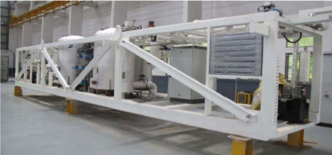
Warm end module that is pre-wired and pre-piped
