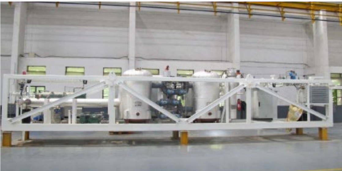
Warm end module that is pre-wired and pre-piped
