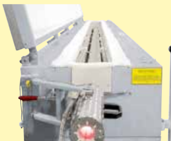
Strand annealing furnaces based on a tube furnace with a length of 6 meters
