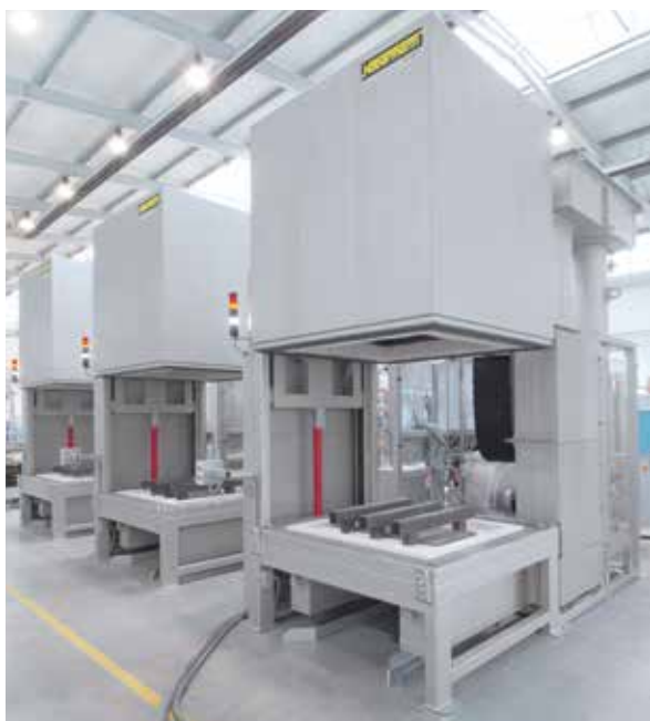
Production plant, consisting of 3 top hat furnaces HAS 1560/95S with sealed housing for operation with nitrogen. Including air/gas heat exchanger for reduced cooling times
