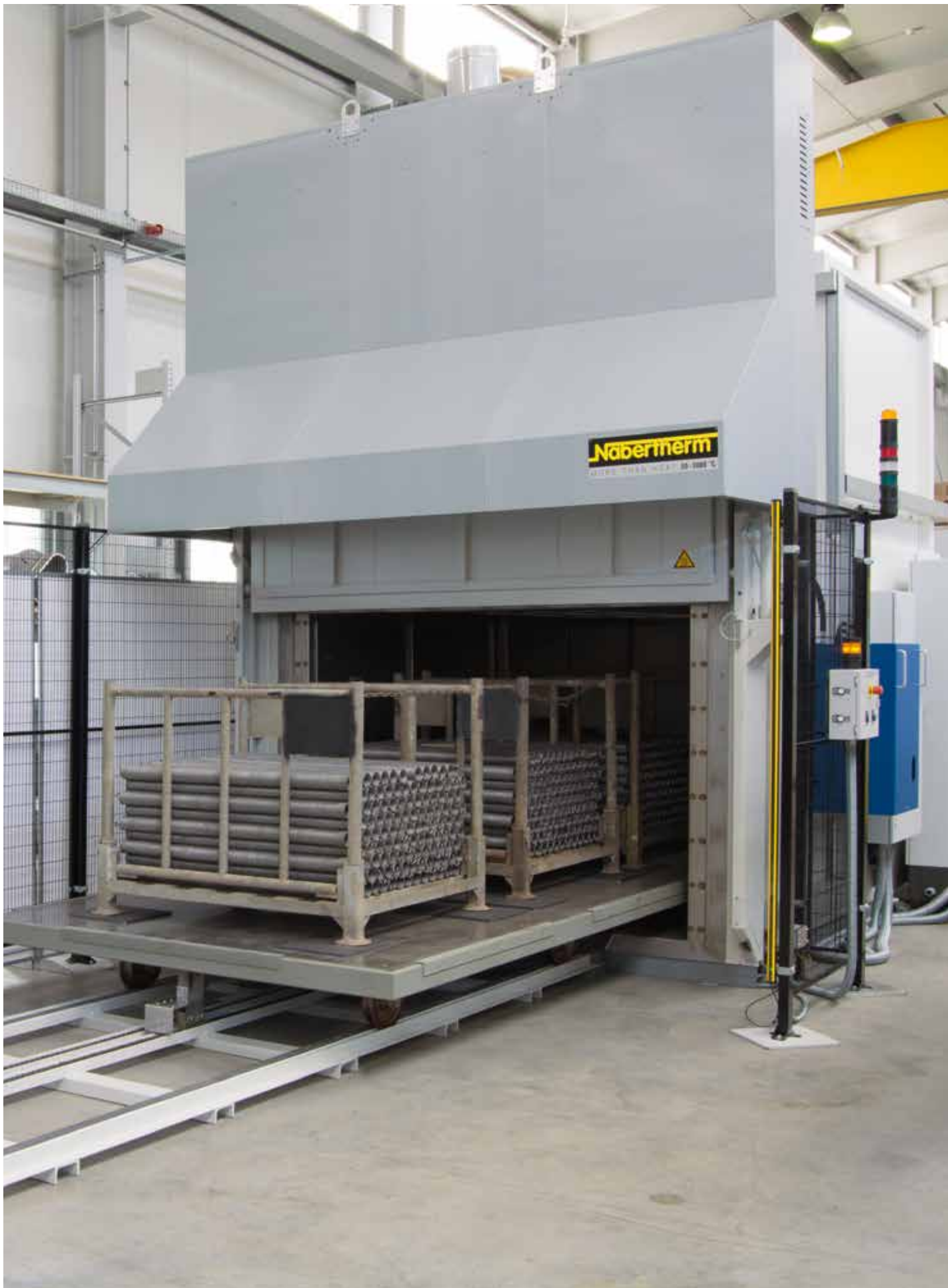
Directly gas-fired forced convection chamber furnace NB 10080/26HAS with driven charging cart
