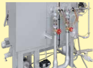
Gas stretch with two burners in the back wall of the furnace
