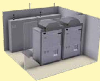
High-temperature furnace with loading from the clean room; switchgear and furnace installed in grey room
