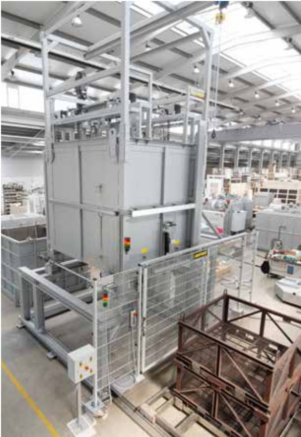
Drop-bottom furnace FS 5670/60AS with quench tank built into the floor (variant C)
