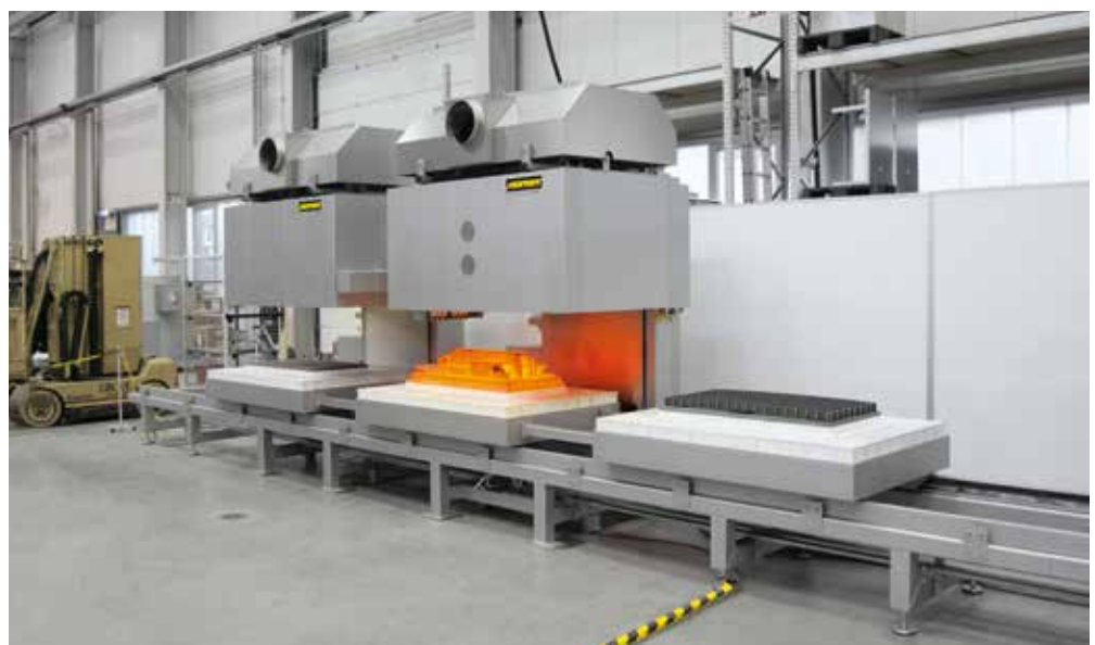
Automatic tempering plant comprising a top hat furnace and two cooling top hats for forced air cooling (the second cooling top hat is on the right not in the picture) with interchangeable table system
