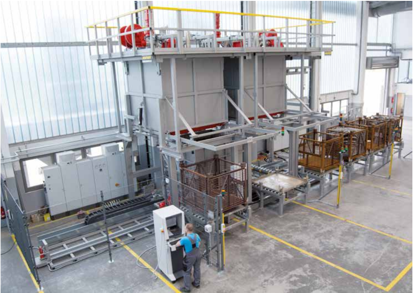
Fully automatic drop-bottom furnace plant, consisting of two drop-bottom furnaces, movable water bath and several loading and unloading positions
