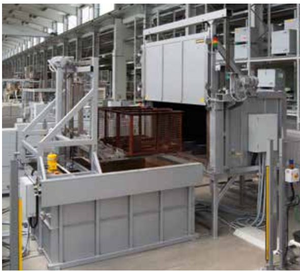
Horizontal tempering plant with forced convection furnace, two-axis manipulator and water quench bath
