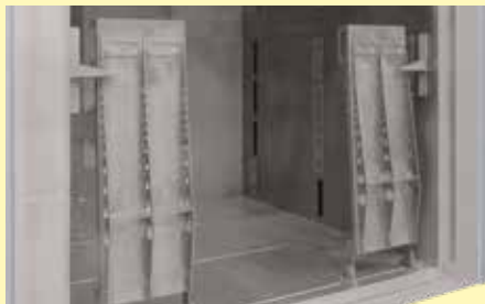
Drive-in ramps at furnaces with bottom insulation for processes which require a good temperature uniformity
