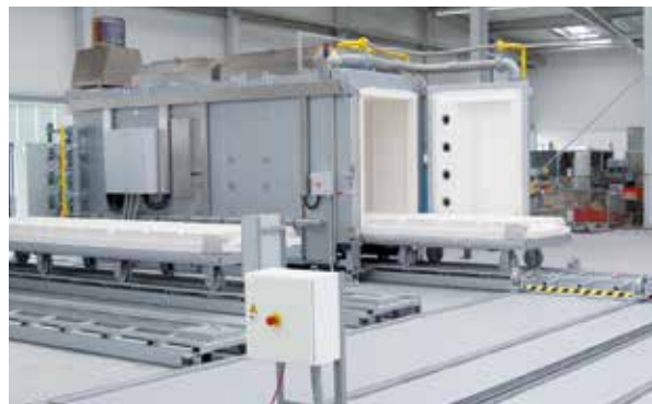
Combi furnace plant consisting of one gas-fired bogie hearth furnace WB 11000/HS and two additional bogies incl. bogie transfer system and incl. necessary park rails
