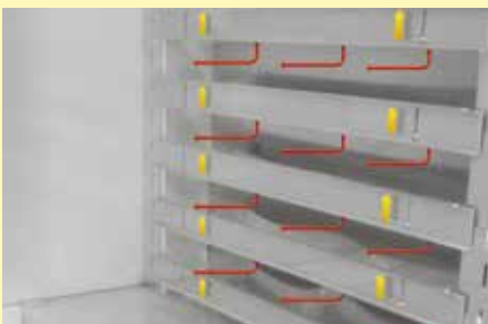
Adjustable plate shutters to adapt the air guide to the charge
