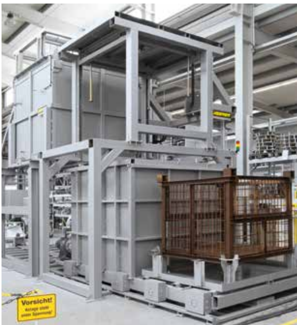
Fully automatic drop-bottom furnace plant with unloading crane (variant B)
