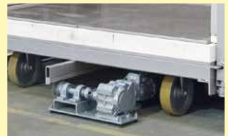
Bogie running on steel wheels with gear rack drive, no rails necessary
