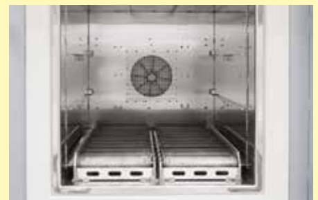
Roller conveyor in furnace chamber
