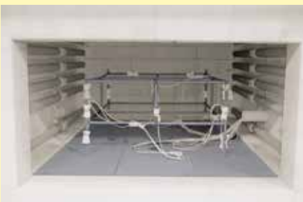
Measurement set-up in an annealing furnace
