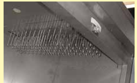
Enclosed heater coils on electrically heated models with Tmax 450 °C and 600 °C
