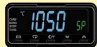
Example of an over-temperature limiter
