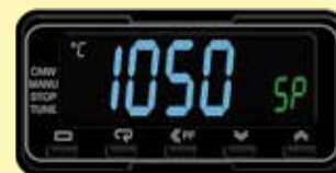
Example of an over-temperature limiter
