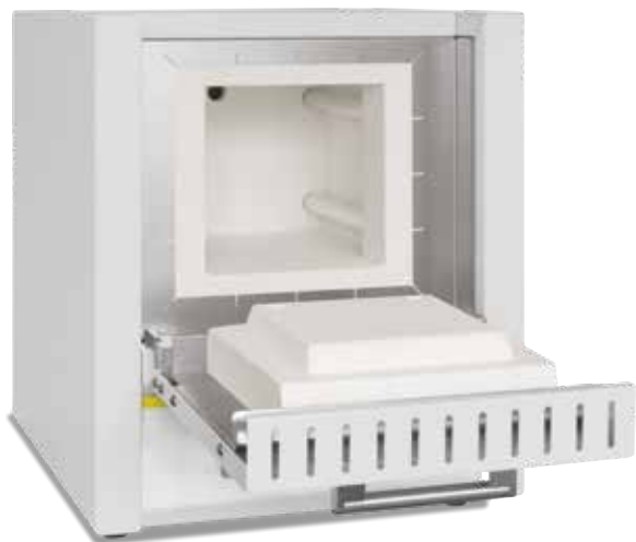
Muffle furnace LE 6/11
