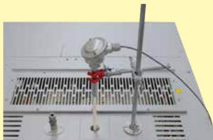
Thermocouple port in the ceiling with tripod
