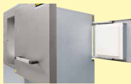
Two-door design for high-temperature furnaces > HT 276/..
