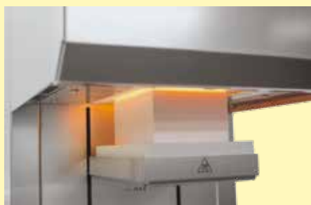
Electrically driven lift-bottom
