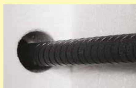
Furnace chamber with high-quality fiber materials and SiC heating rods on both sides of the furnace
