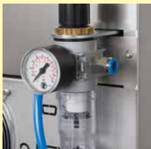
Forced cooling system with compressed air
