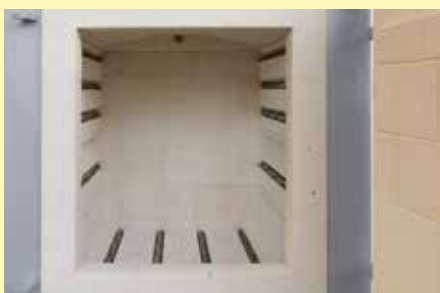
Three-sided heating with heating elements protected in grooves
