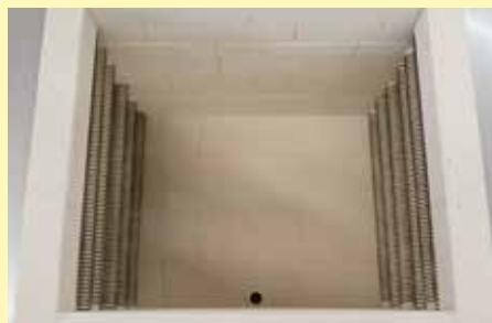
Heating elements on support tubes ensure uninterrupted heat radiation
