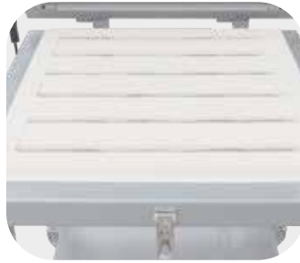
Floor heating provides for even heating of larger objects
