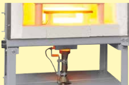
15 kW propane gas burner mounted under the kiln
