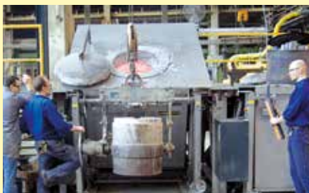
Charging of transport ladle with tilting furnace K 360/12
