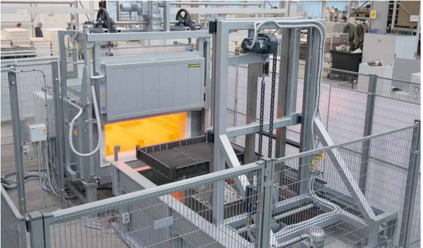
Automatic quenching and tempering plant N 644/S
