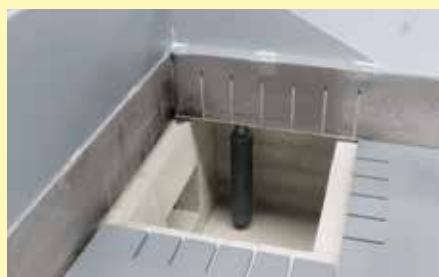
Melting thermocouple in the bath of the outlet opening
