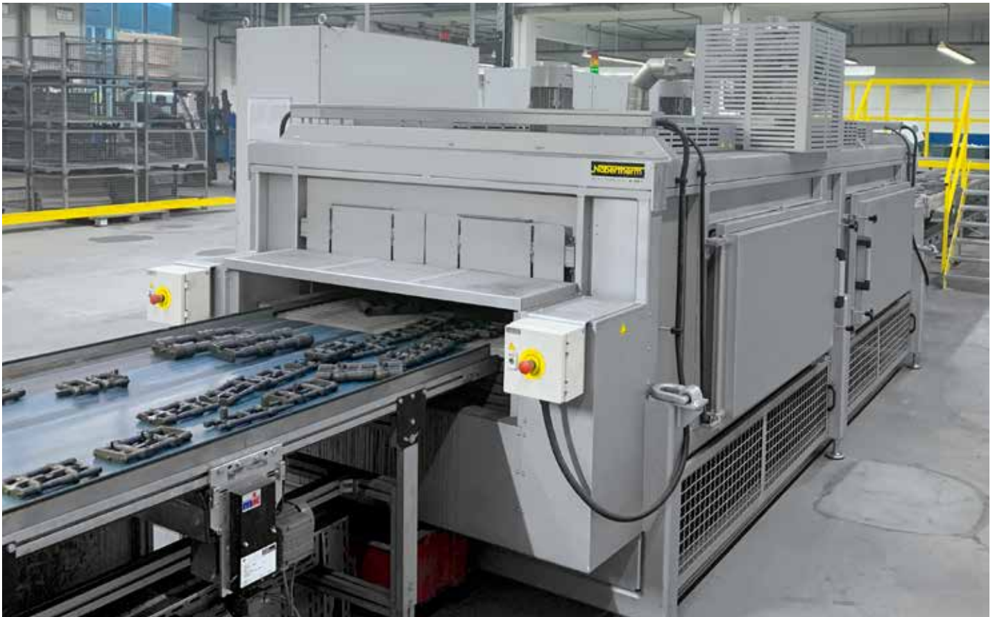
Continuous belt furnace D 1000/4000/140/35 AS for black wash drying on sand cores
