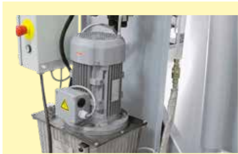
Hydraulic system with flame resistant hydraulic fluid
