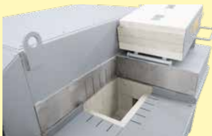
Inlet opening for filling with liquid aluminum
