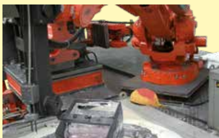
Bale-out of bale-out furnace with robot
