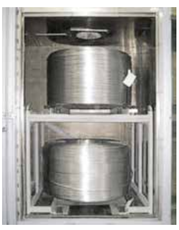
Heat transfer between a hot and a cold charge
