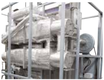
Counterflow heat exchanger for the forced convection chamber furnace N 2560/26 ACLS
