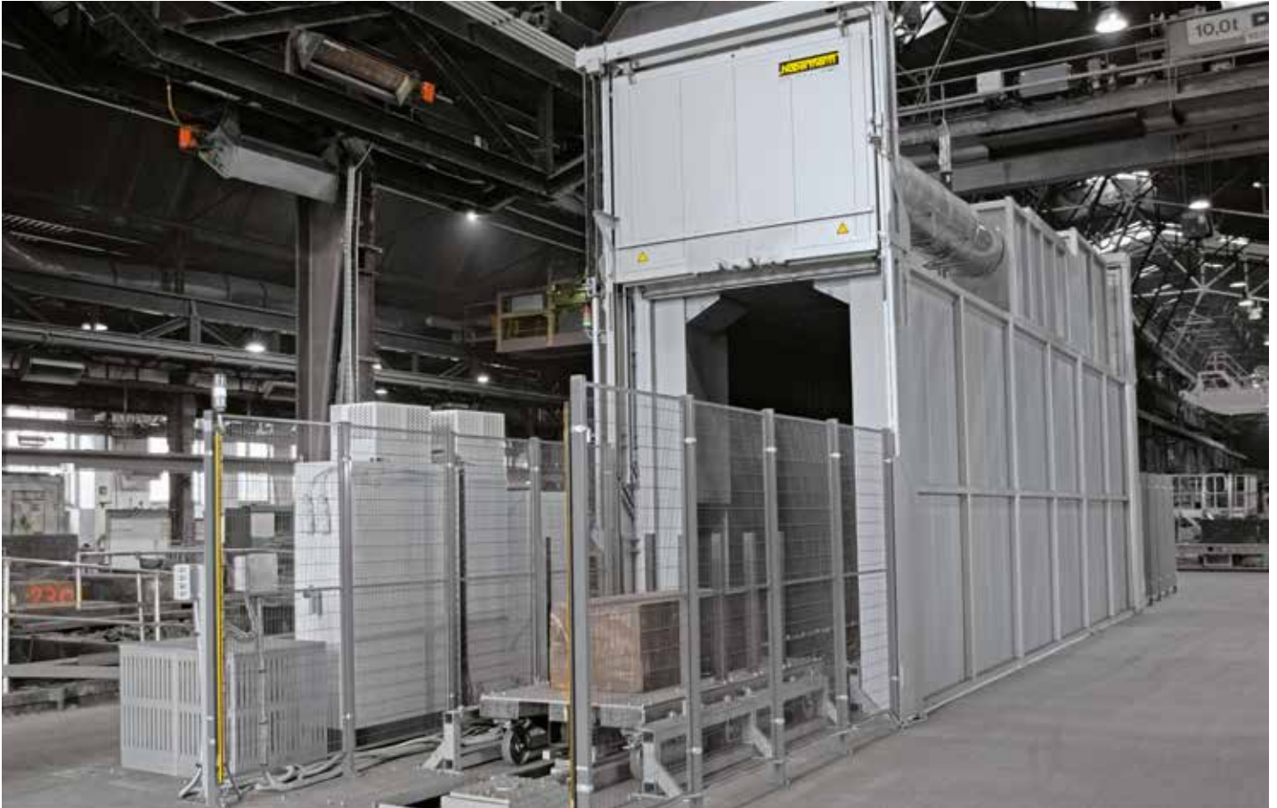
Continuous pilgrim step furnace system NBI 70000/15HAS for black wash drying on sand cores
