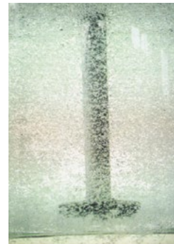
Dispersion of Gas (Water model)
