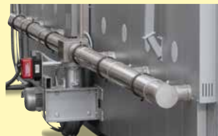
Cooling system with fresh air fan
