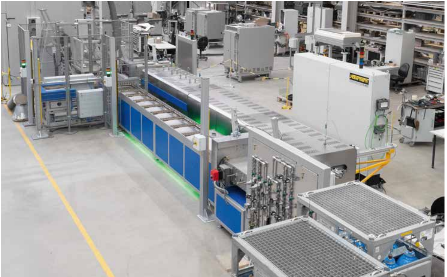
Pusher-type furnace system D 520/2600/55-04 S to sinter teflon coatings under protective atmosphere
