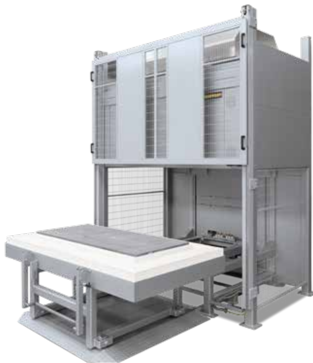
Bottom loading furnace HF 1220/LBS with fiber insulation, safety barrier to safeguard the danger zone and manually movable table for ease of loading and unloading
