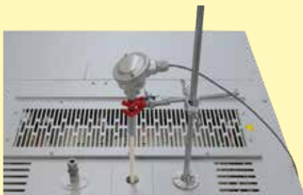
Thermocouple port in the ceiling with tripod
