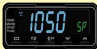
Example of an over-temperature limiter
