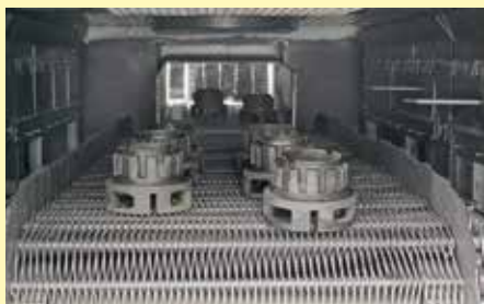
Mesh belt drive in a continuous furnace
