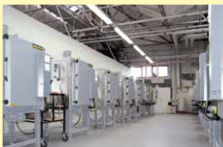
Chamber furnaces N 200/14 for sintering semiconductors
