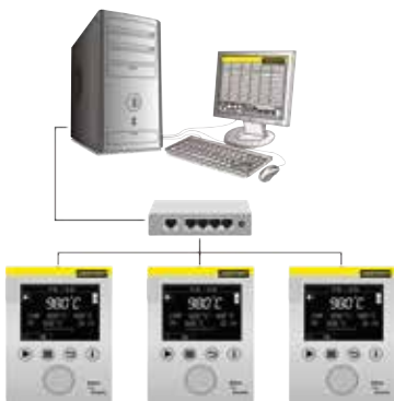
Example lay-out with 3 furnaces
