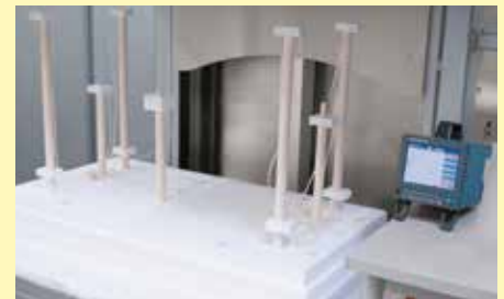
Measurement setup to determine the temperature uniformity in a high-temperature bottom loading furnace
