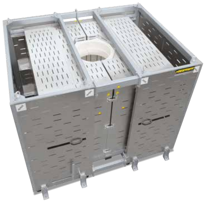
Split-type tube furnace RSV 460/1000/16S for vertical operation
