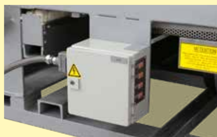
Charge thermocouples with plug-in connection
