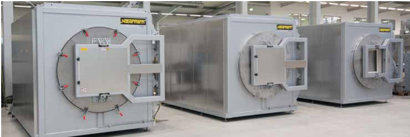
Hot-wall retort furnaces NR 1000/11 in production
