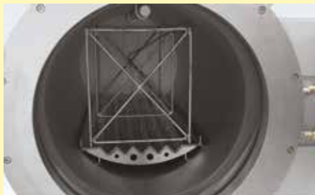
Charging support and TUS measuring frame for retort furnace NR 20/11
