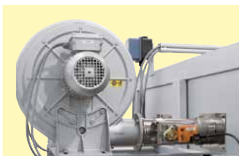
Cooling fan for accelerated cooling
