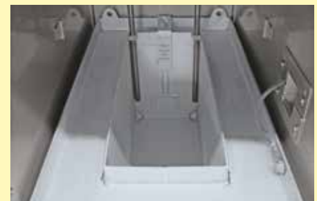
Crucible made of high-quality CrNi steel
