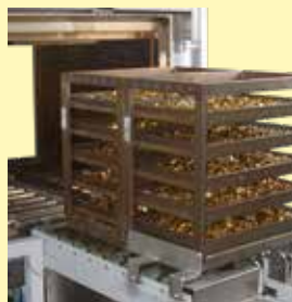
Continuous furnace for bulk materials in baskets
