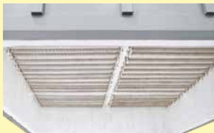
Heating elements in furnace hood
