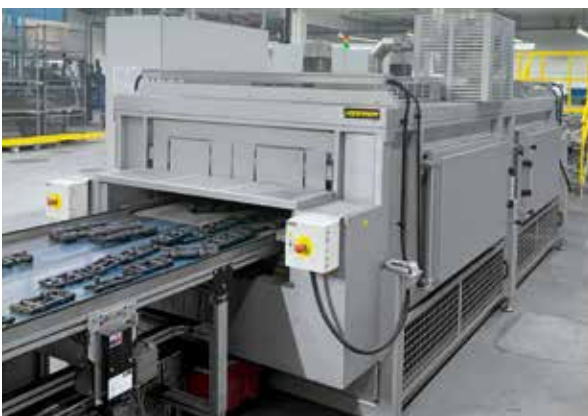
Continuous belt furnace D 1000/4000/140/35 AS for black wash drying on sand cores
