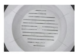
The amount of treatment can be changed (modified) to "30 kg or less" or "50 kg or less" by reinforcing the bottom. A heavy object can be treated in this case.
