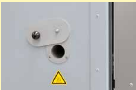
Port for thermocouple
