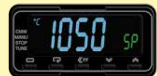
Example of over-temperature limiter
