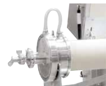
Water-cooled vacuum flange (gas supply system 2)
