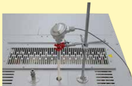
Thermocouple port in the ceiling with tripod
