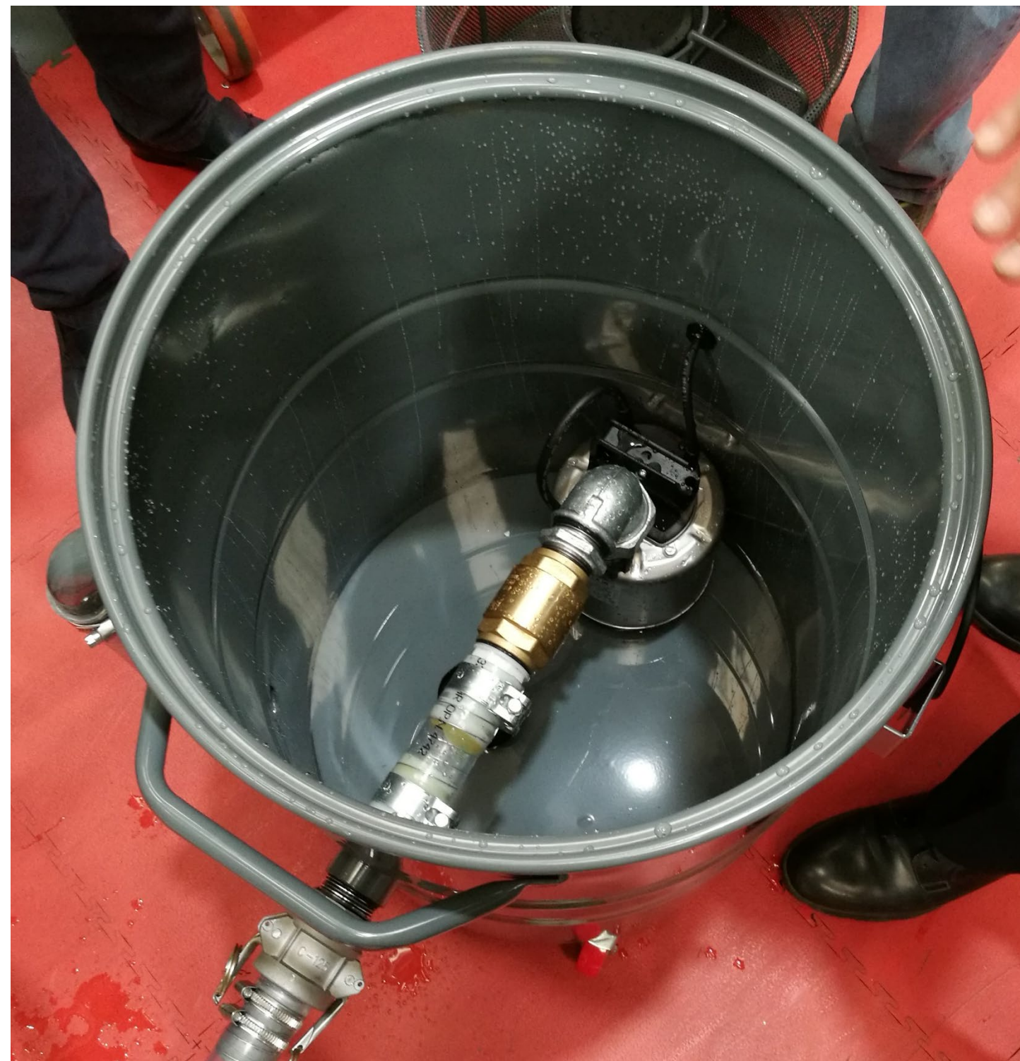
Discharge pump 140 lt/min
