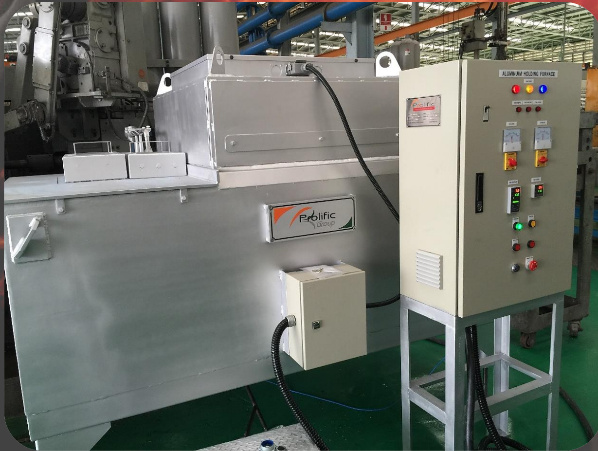
Aluminum Holding Furnace Capacity 300 Kg/hour
