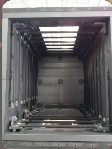
Repair insulation and heater of vacuum furnace
