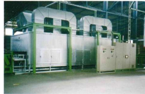
Continuous jet-nozzle hot-air oven for preheating building materials
