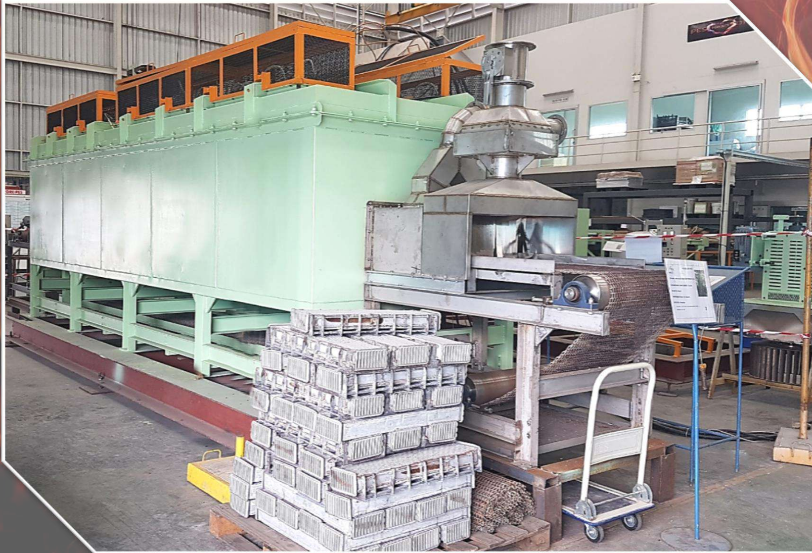
Dry Off Furnace/Mesh Belt Type Maximum Temperature of 350 C
