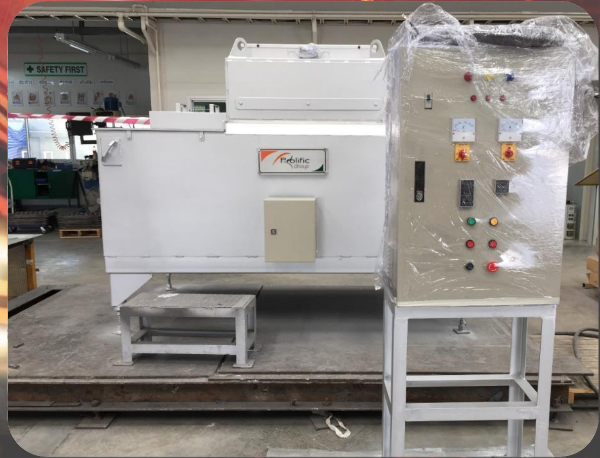
Aluminum Holding Furnace Capacity 300 Kg/hour
