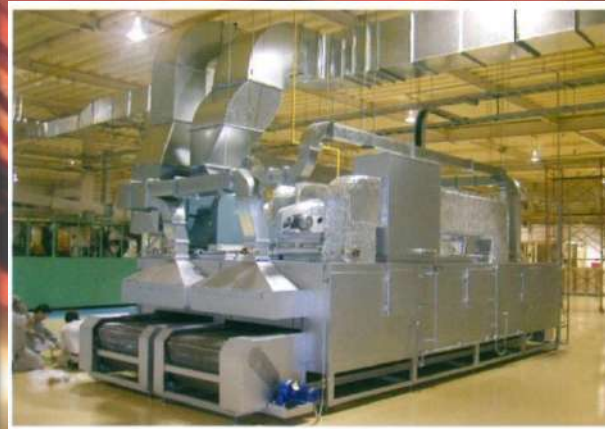
Continuous conveyor oven for auto plastic parts
