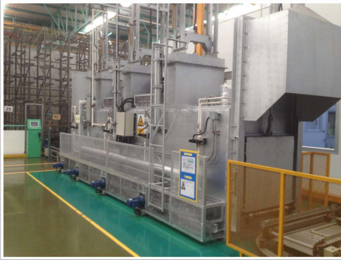
Continuous direct hot-air / far-infrared oven for painted engine parts
