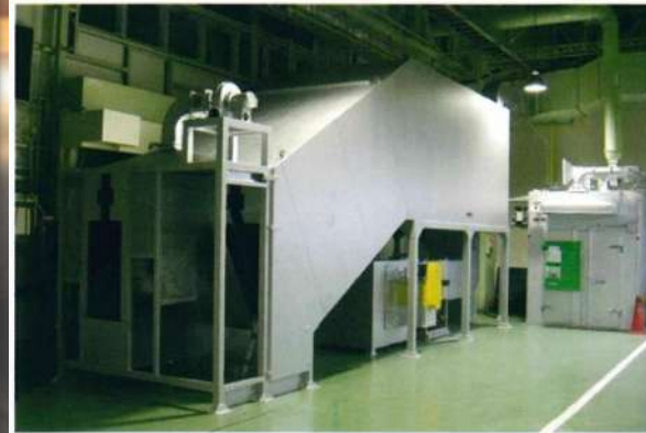
Continuous direct hot-air / far-infrared oven for painted engine parts
