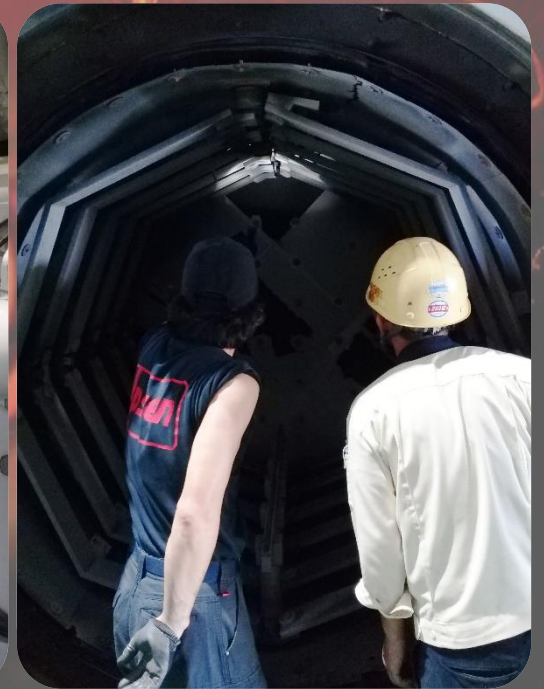
Helium leak testing and repair insulation in vacuum furnace
