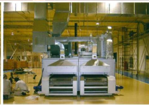
Continuous conveyor oven for auto plastic parts
