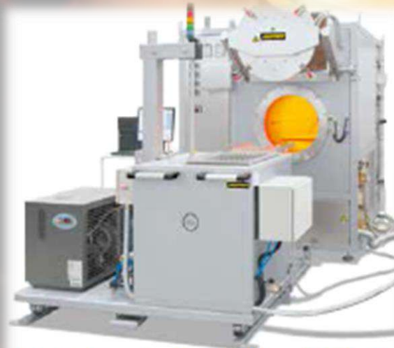
Semi-automatic annealing plant with retort furnace NR 5Q/11 and water quenching bath on rails
