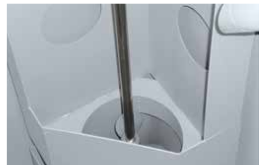
Circulation of quenching medium
