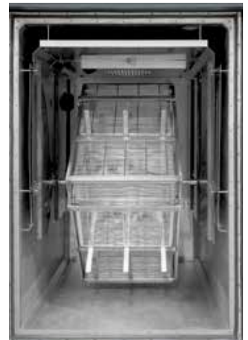
Motor-driven rotary rack with baskets for moving the charge during heat treatment
