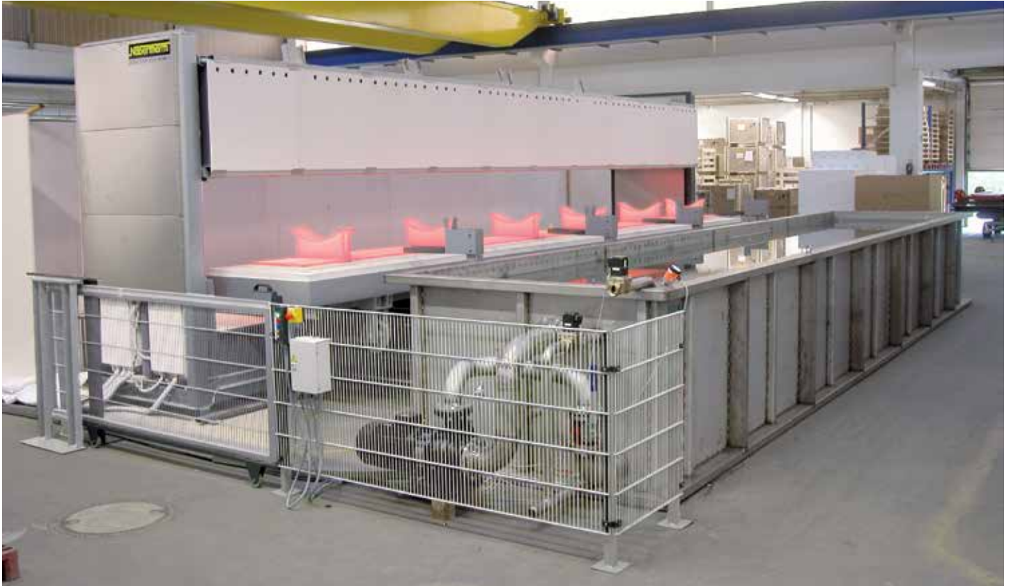
Tempering plant with top hat furnace H 4263/12S and water bath
