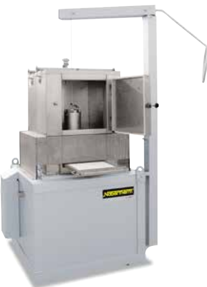
Salt-bath furnace TS 30/18 with preheating chamber above the salt bath and charging aid for immersion of the charge
