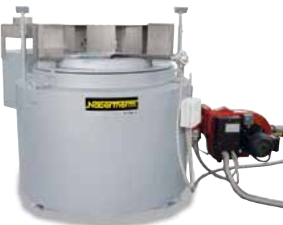
Salt-bath furnace TSB 30/30, gas-fired
