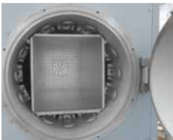
Inside heating in retort furnace NRA ../06
