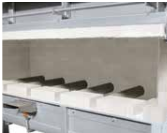
Indirect gas firing with radiation tubes
