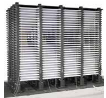
Kiln furniture for small ceramics components
