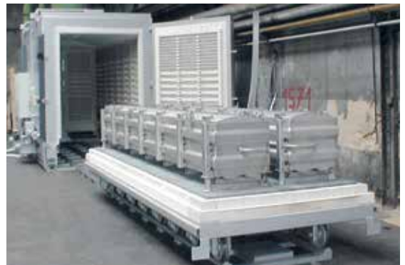
Bogie hearth furnace with gas supply system
