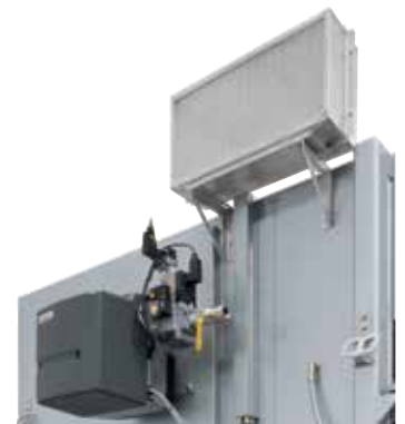
Direct gas-firing at a chamber dryer
