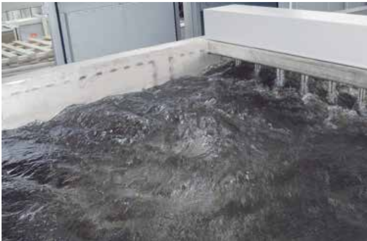
Powerful circulation of quenching medium
