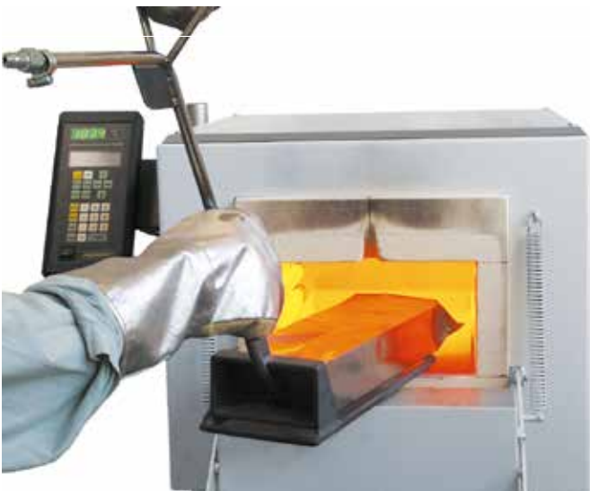
Hardening in annealing tray with alloy bag
