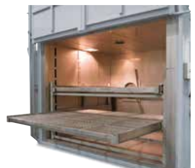
Pull-out drawers for heavy loads
