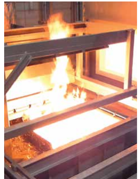
The charge is placed in the hot furnace by a manipulator and is also removed and transferred to the quenching medium while it is hot.
