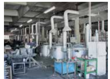
Recuperator burner for aluminum melting furnace 16 x TBR 110/12 and 2 x TBR 180/12
