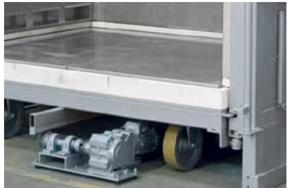
Bogie running on steel wheels with gear rack drive, no rails necessary
