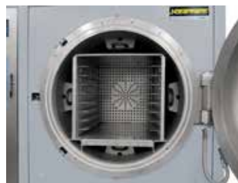
Retort with internal heating and process chamber
