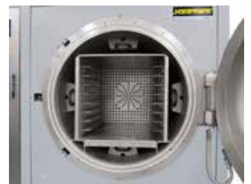
Retort with internal heating
