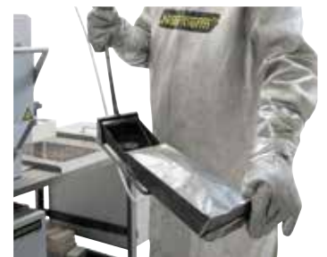
Protective gas annealing bag in operation
