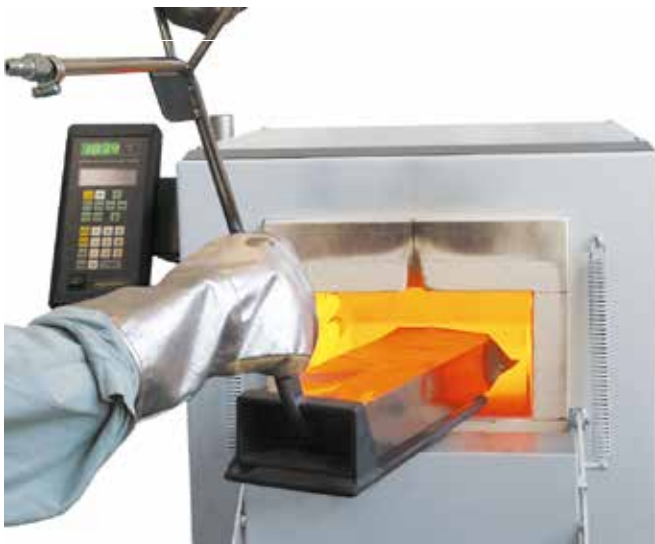
Hardening in annealing tray with alloy bag
