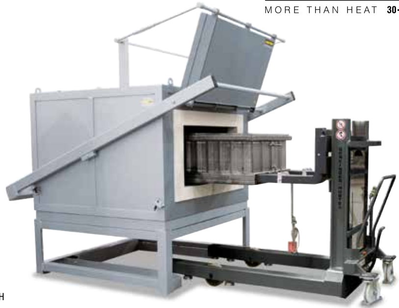
Chamber furnace N 321 with charging stacker
