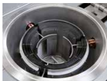
Cylindrical retort with tungsten heating
