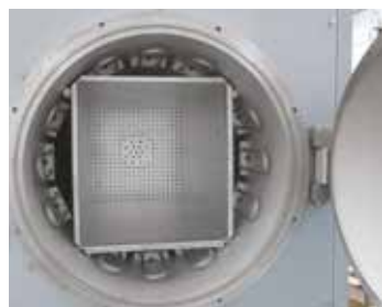
Inside heating in retort furnace NRA ../06
