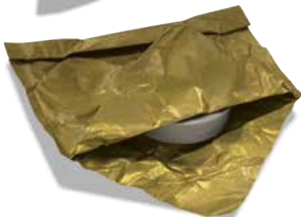
Workpieces in foil heat treating
