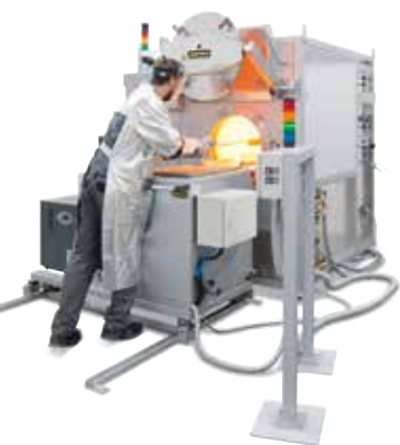
Semi-automatic annealing plant with retort furnace NR 50/11 and water quenching bath on rails
