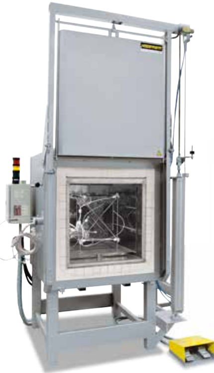
Holding frame for measurement of temperature uniformity
