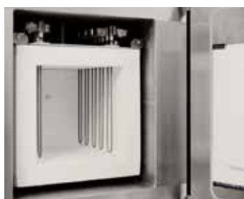
Molybdenumdisilicide heater and fiber insulation
