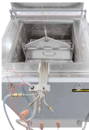
Protective gas box, AMS 2750 E design
