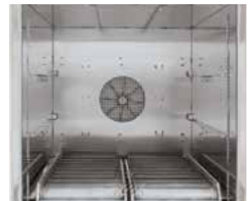
Roller conveyor in forced convection chamber furnace N 250/85HA
