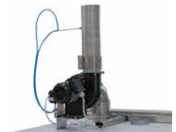
Exhaust port and powerful exhaust fan mounted on the furnace
