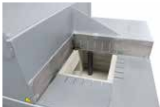
Melting thermocouple in the bath of the outlet opening
