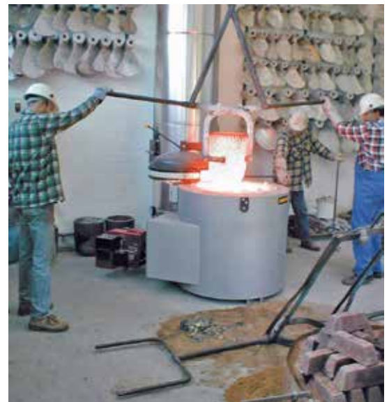
Bale-out furnace TB 20/14 for bronze melting with side exhaust gas discharge and swiveling collar plate for crucible pulling
