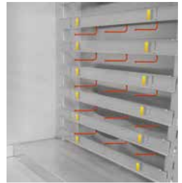
Adjustable plate shutters to adapt the air guide to the charge
