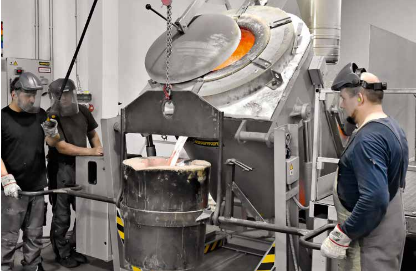
Tilting furnace KB 150/12 in production
