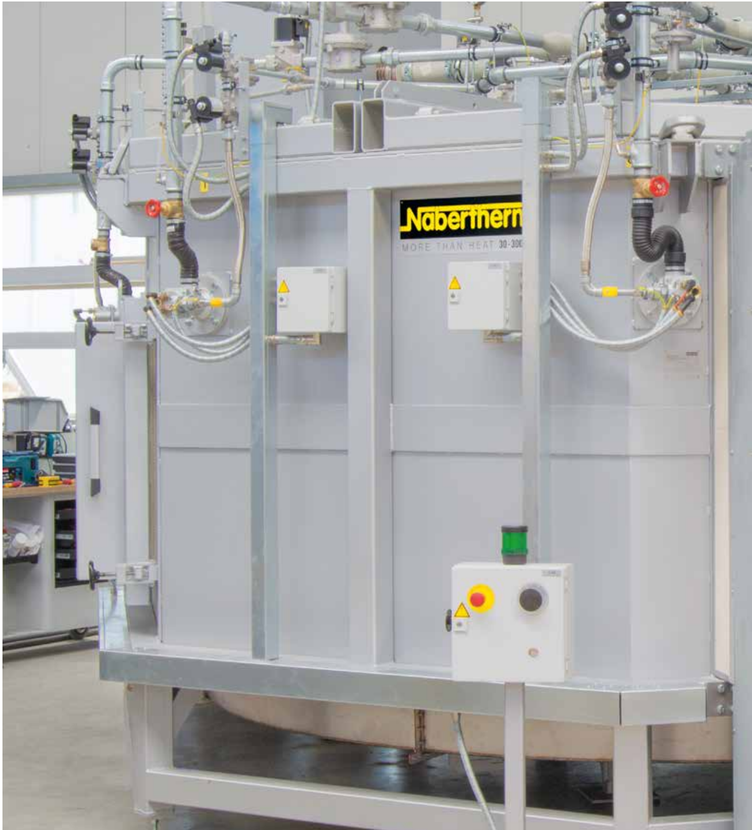
Gas-fired rotary-hearth furnaces for preheating of ceramic moulds up to 1100 °C incl. thermal post combustion for exhaust gas cleaning
