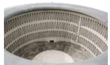
Meander heating elements
