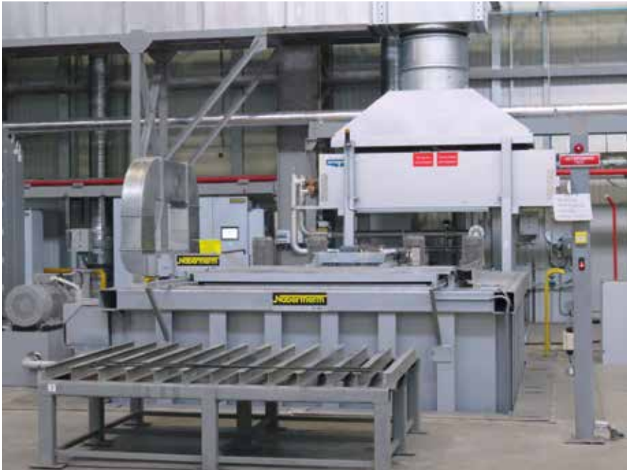
Oil quenching bath OAB 67000 with heat exchanger and a volume of 67.000 liters oil
