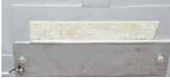
Crucible breakage alarm device under the emergency outlet of a melting furnace
