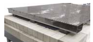
Charge support made of perforated sheet metal
