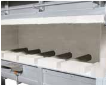
Indirect gas firing with radiation tubes
