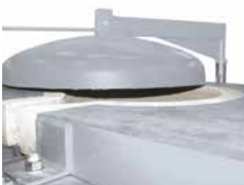
Swing lid with good sealing to collar plate to avoid heat loss over the crucible opening
