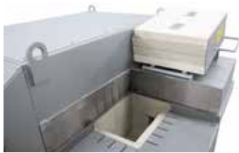
Inlet opening for filling with liquid aluminum
