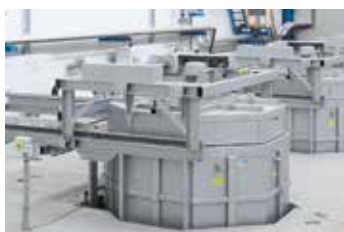
Forced convection pit-type furnaces S 10400/75 AS in production
