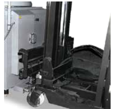
Slots under the furnace for the forklift forks
