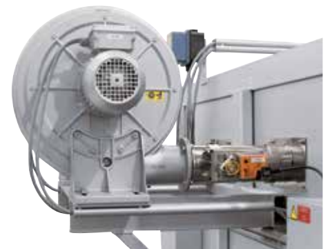
Cooling fan for accelerated cooling
