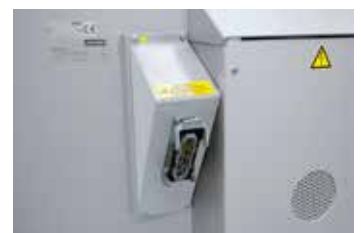
Plug socket on the furnace for the cable connection to the switchgear and control box
