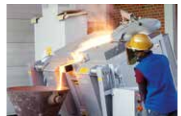
Tilting furnace KC 80/14 during casting
