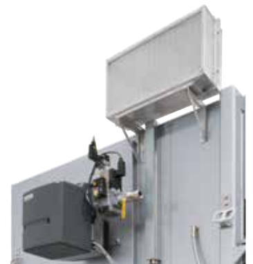
Direct gas-fired at a chamber oven
