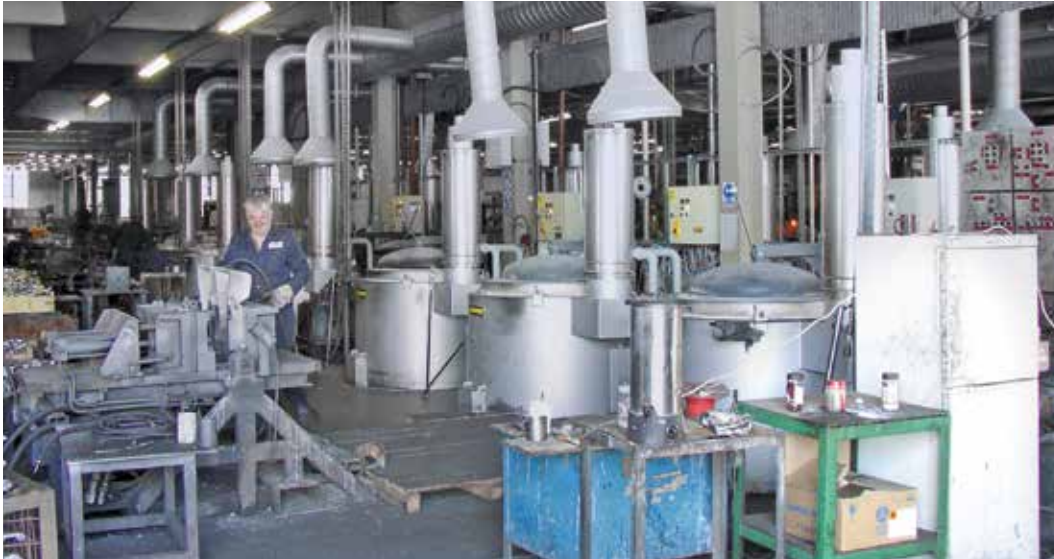
Production with 16 crucible furnaces TBR 100/11 and 2 crucible furnaces TBR 180/11
