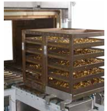
Continuous furnace for bulk materials in baskets
