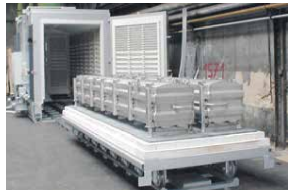
Bogie hearth furnace with gas supply system
