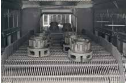
Mesh belt drive in a continuous furnace
