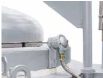
Thermocouple for melt bath control
