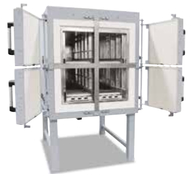
Forced convection chamber furnace NA 500/45S with four compartments, each with roller conveyor and individual door
