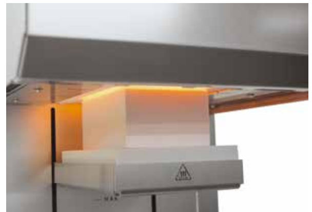
Automated table lowering for cooling
