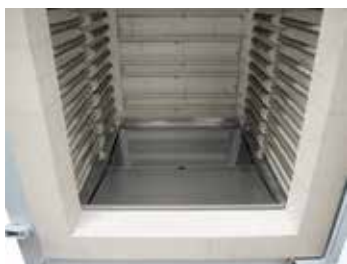
Drain pan in floor
