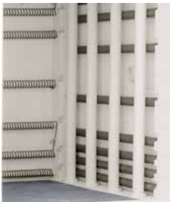
Injection of preheated air through perforated ceramic tubes
