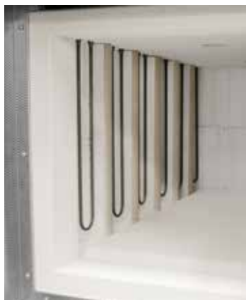
Protection of heating elements against mechanical damage
