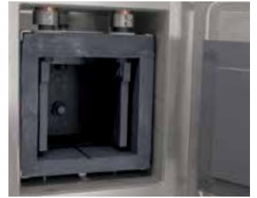
Graphite heating chamber
