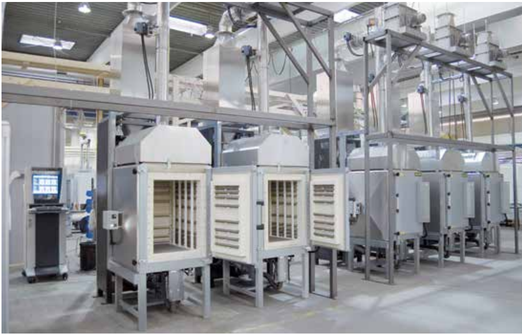
Production system consisting of five combi chamber furnaces N 300/H DB200 with catalytic afterburning
