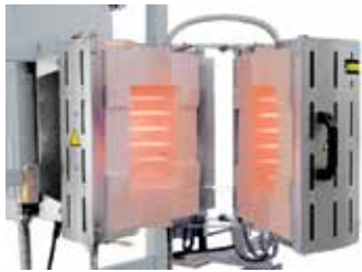
RS 100/250/11S in split-type design for integration into a test stand
