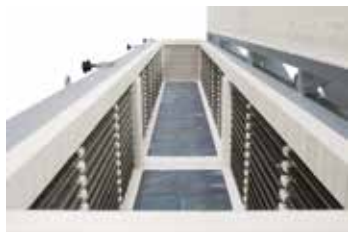
Furnace chamber S 5120/GS with receptacle for an insulating plate in order to divide the furnace chamber
