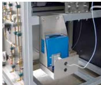
Acid pump for nitric acid
