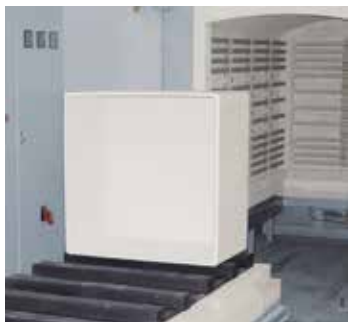
Bogie hearth furnace W 3300 for glazing melting crucibles for the solar industry
