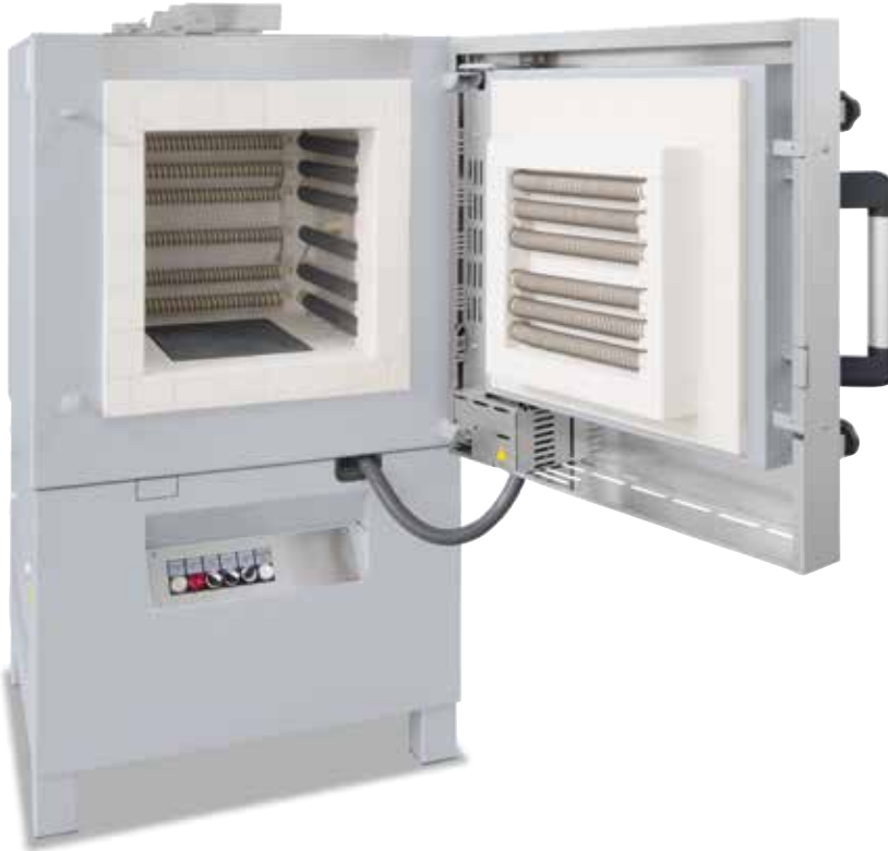
Chamber furnace LF 60/14 with fresh air fan to accelerate the cooling times
