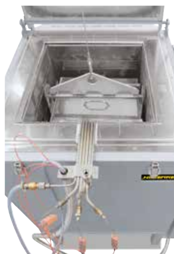
Protective gas box, AMS 2750 E design
