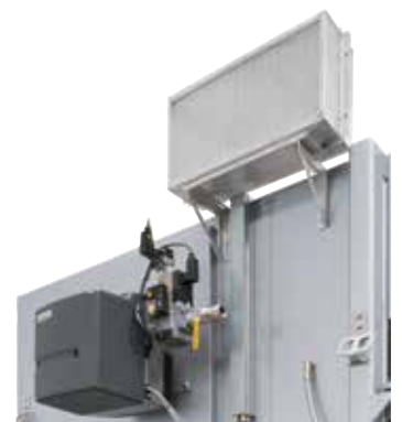
Direct gas-firing at a chamber dryer
