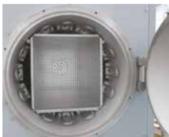
Inside heating in retort furnaces NRA ../06
