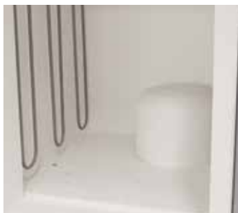
Inner process top hat with gas injection through the furnace bottom protects the furnace chamber against contamination and/or prevents chemical interaction between the charge and heating elements
