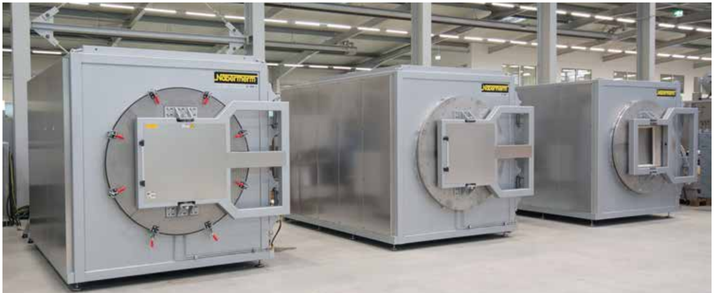
Hot-wall retort furnaces NR 1000/11 in production
