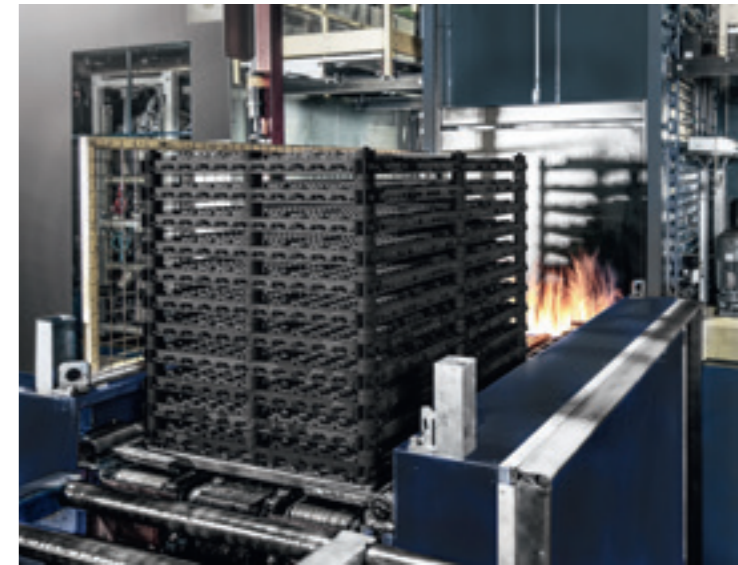
↑ Multi-layer CFC fixture in use
