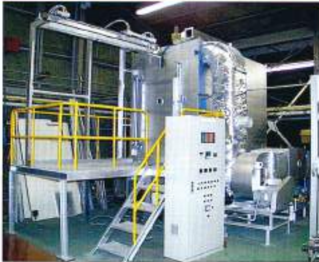
Testing furnace at our Kanagawa Factory Far-infrared burner BT-33NH x 4 units
