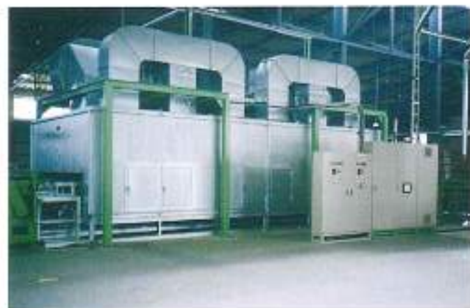
Continuous jet-nozzle hot-air oven for preheating building materials
