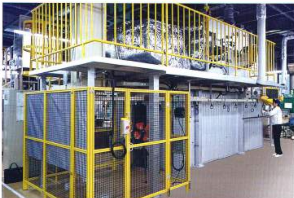
Metallic parts jet hot air painting furnace (slit nozzle type) Indirect hot air type (Radiation amount 152 kW) Max. gas consumption LPG 12.5kg/h, 13A 14.0m 3 /h
