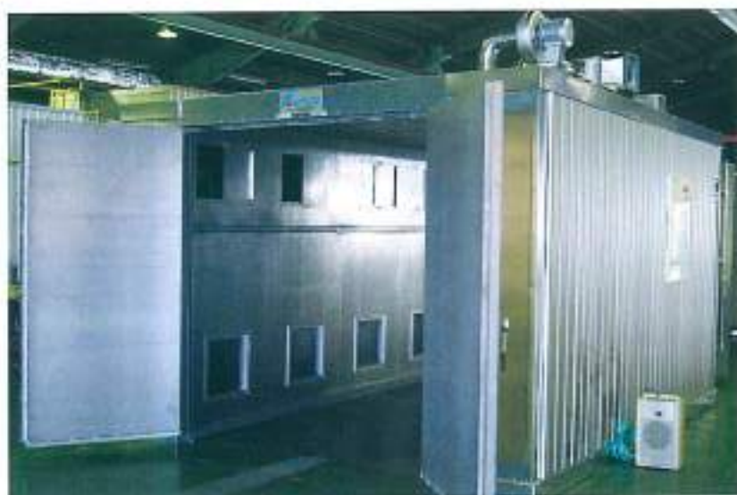
Solvent coating, New batch furnace equipped with PWT
