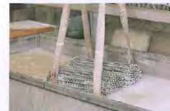
7 脱脂洗浄 Degreasing
