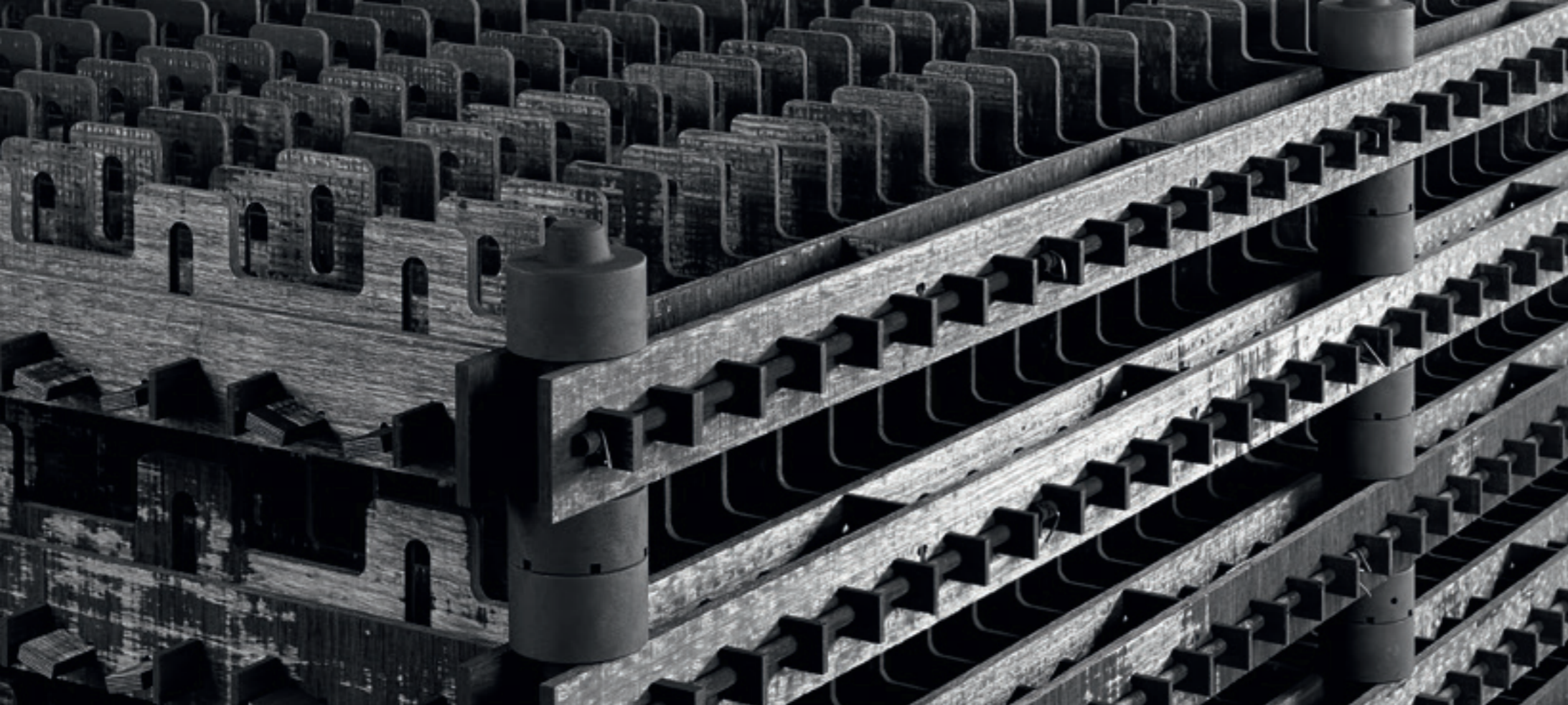
↑ CFC workpiece fixtures for gas carburizing with oil quenching, stackable.
